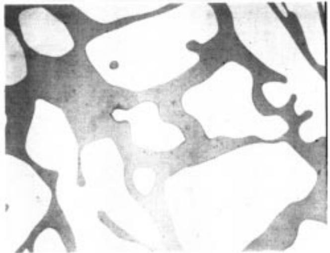
FIG. 2 (a) J92205: Unaffected Structure-Statically Cast (400× Magnification)
